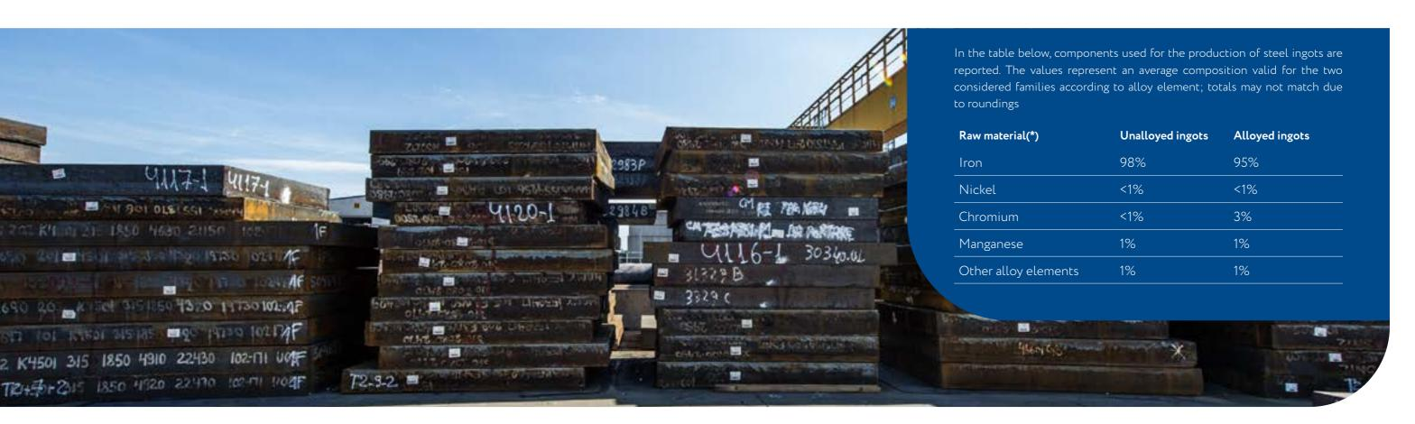
OBJECT OF THIS EPD® IS THE FAMILY OF STEEL INGOTS PRODUCED VIA EAF TECHNOLOGY.
